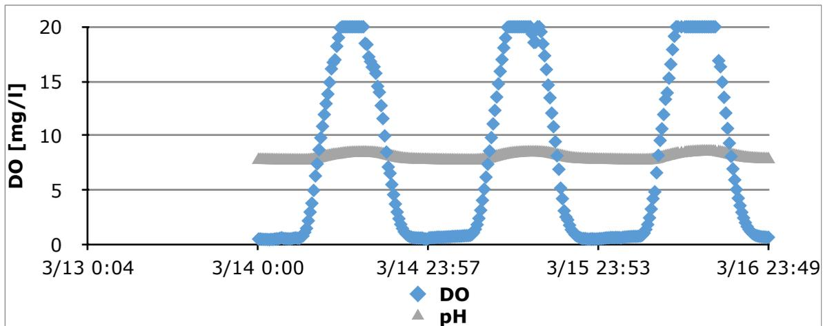
**Figure 4: Fluctuating dissolved oxygen concentration and pH from day to night in beta site raceways.**
