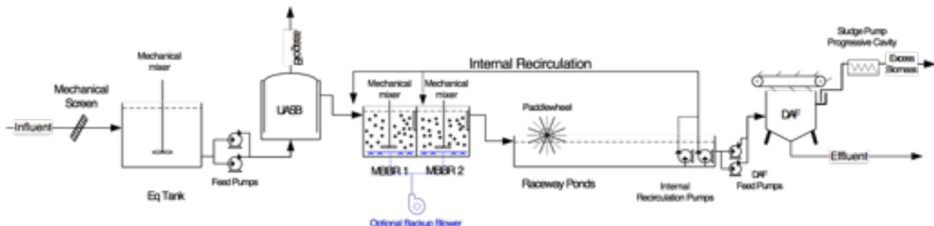
Following harvesting of algal solids, DAF effluent meets TSS, COD, BOD (and nutrient, where applicable) discharge targets.
